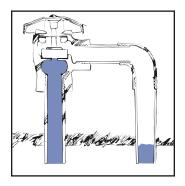
In this view of a double check valve, there is backpressure from a source downstream which has caused the second check to close tightly against this reverse pressure. The first check has closed tightly by itself, thus giving two barriers against the backflow condition.
