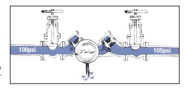
In this view of a pressure vacuum breaker, a backsiphonage condition has caused the check to close against its seat and the air-inlet has opened so that the pressure in the body of the device is atmospheric. If the check was fouled by some foreign material, only air would be pulled back into the domestic supply system instead of the non-potable water downstream of the device.
