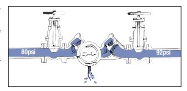
In this figure of an RP device, there is a backpressure condition. The second check is fouled with a piece of pipe scale which permits the higher pressure to flow back into the zone. Here the relief valve discharges the water to atmosphere maintaining the pressure in the zone lower than the supply pressure.
